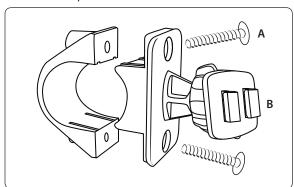
Step 3. Wrap the rubber rings (C) around the handlebar and reassemble the ball plate and swivel head (B) around the rubber rings. Secure the mount assembly by using the screwdriver to retighten the two mounting screws.
